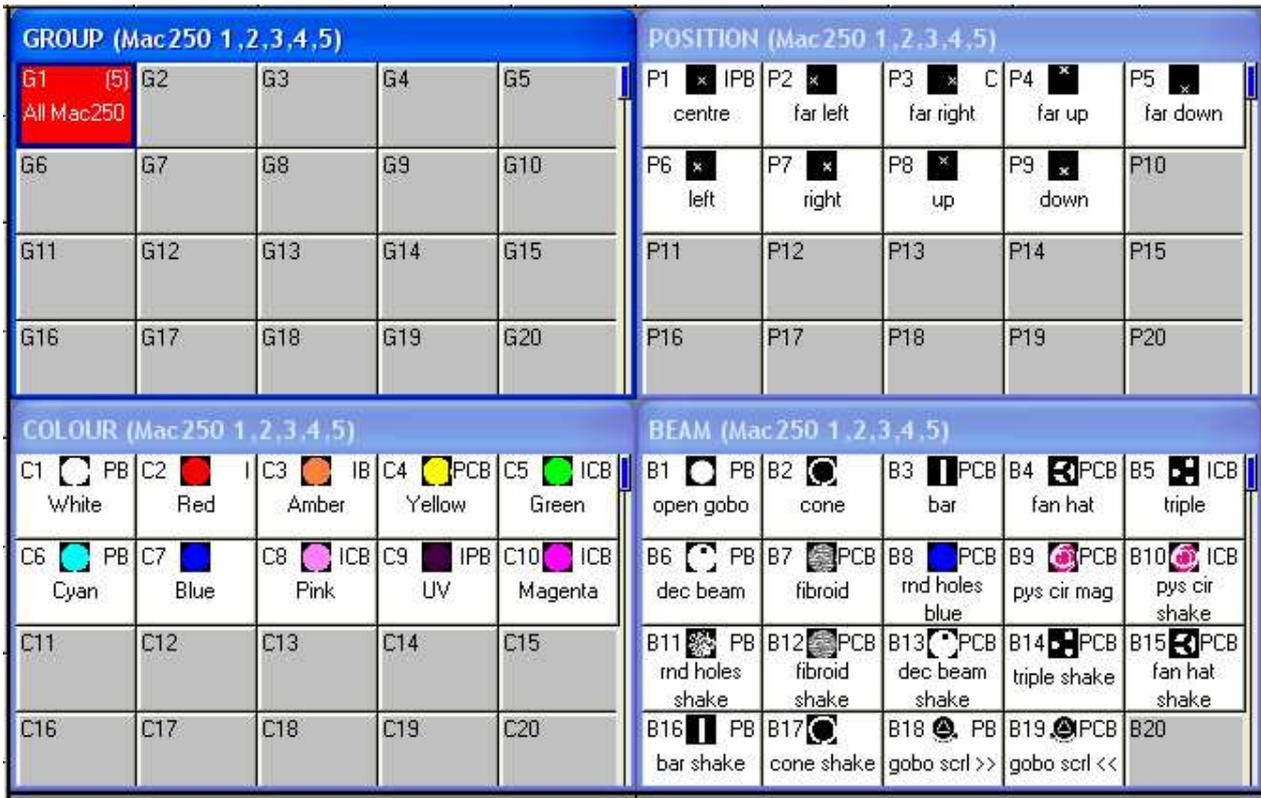
In the Colour Window there is a COL MIX soft button which gives access to libraries of pre-programmed colours. Pressing the COL MIX soft button toggles between the normal palette view and the colour mixing view. In the colour mixing view you can select a colour using the touch screen. The COL TYPE soft button enables the user to choose between the default colour library, the Lee colour library or the Rosco colour library.
