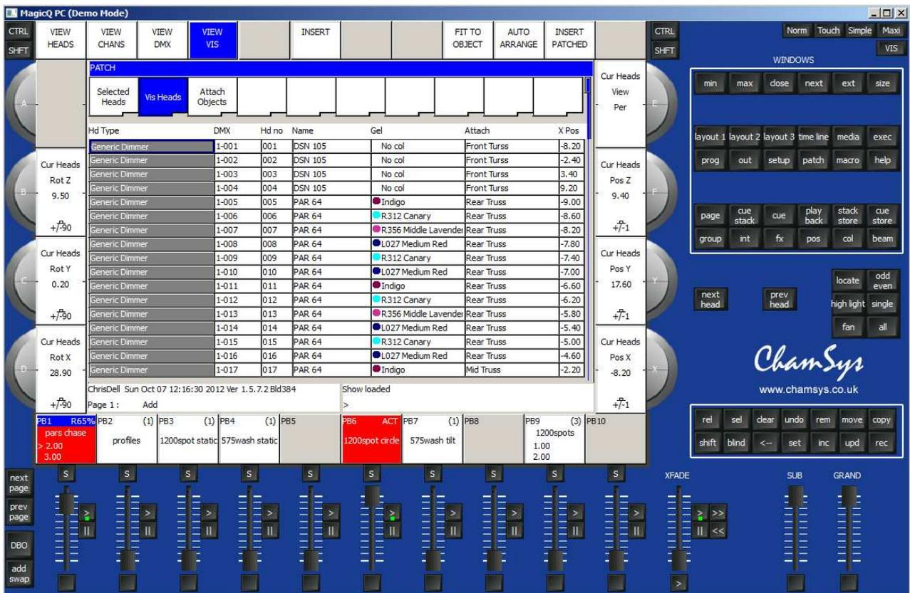
In Selected Heads, all the visualiser heads for the currently selected heads will be shown in the list. Heads are selected as usual using groups or direct from the keypad. In this view the encoders and soft buttons will apply changes to all the visualiser heads for the selected heads.
