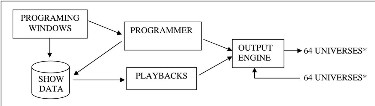
\* 64 universes except MQ40 (4), MQ60 (12), MQ70 (12), and MQ100 Expert (12). Older consoles such as MQ Pro support 18 and MQ Pro 2010 supports 32.
