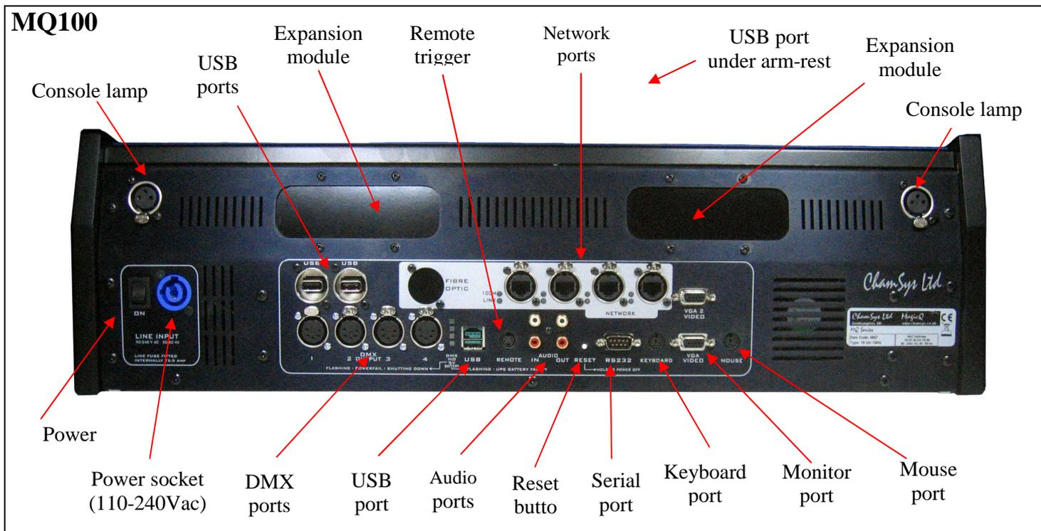
MagicQ MQ100 Expert consoles have a similar rear panel but with only one network port and two (non locking) USB ports. MQ100 Expert consoles do not have VGA ports for additional monitors.
