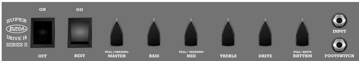
**On/Off:** Power On and Off switch. Make sure the black Go/Rest switch is set on Rest before you turn the power to On.
